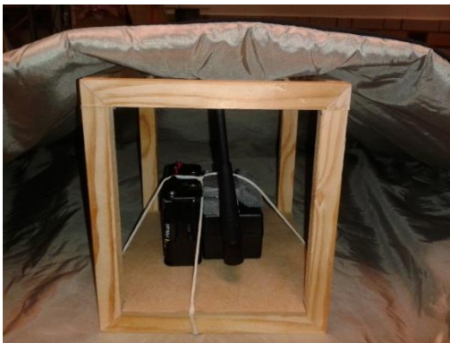
Fig. 3: Showing the comb completely covered by the Faraday bag
