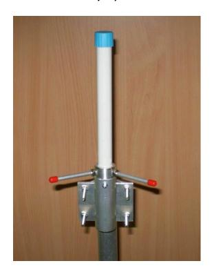
Antenna omni-directional 360°, very rugged construction mounting secured by strong AL holder with 2x M5 stainless steel bolt. Pole diameter up to 55mm. Antenna radome material is polycarbonate.
