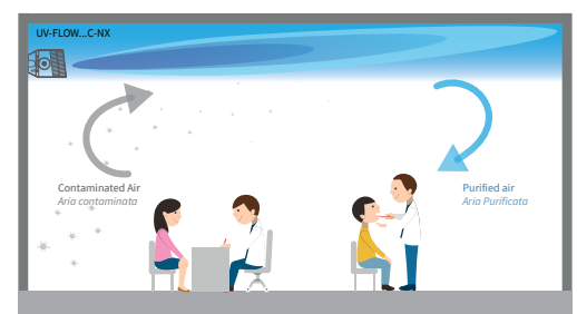
Disinfection of air upper layers
