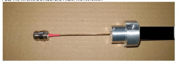
MEASURE WITH THE APPROPRIATE TOOL THE ELEMENT LENGHT AND CUT ACCORDING THE CUTTING CHART, POSITION THE METER AT THE POINT WHERE THE CONNECTOR ENDS AND ELEMENT BEGIN, USE PERNAMENT MARKER TO MAKE THE DOT ON THE ELEMENT
