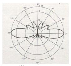
This manual is for collinear antenna 868mhz / 5Dbd gain
