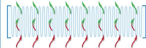
Phase 3: The **Final Filter AC Pleated** adsorbs unpleasant odours and gases. Finally a **Silver Ion filter** and **UV-C light** solution are added to kill off remaining airborne viruses and bacteria.
