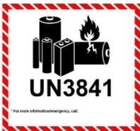
Lithium polymer batteries contained in equipment or packed with equipment.
