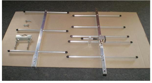
SLIDE THE 3 ELEMENT PART TO THE MAIN PART, OBSERVE THE ELEMENT SCREWS TO MATCH THE OTHER, USE SOME FORCE IF NECCESARRY AND ALLING SCREW HOLES, USE ENCLOSED SCREWS TO SECURE THE BOOM AND TIGHT STRONG. THE PROCEDURE IS REPEATABLE AND ANTENNA DOES NOT SUFFER BEING REPAETABLY ASSEMBLED WHAT IS A GOOD FEATURE FOR FIELD OPERATIONS. IN RARE OCCASIONS, ANTENNA CAN BE USED WITHOUT ADDITIONAL 3 ELEMENT SECTION.
