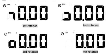
Every rotation should trigger the segment – if not, please check your wheel sensor position. This testing segment will show up always after resetting the trip. This serves also as an indicator of the zero position (no rotation was made, start of special stage).
